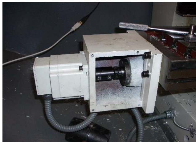
Figure 9.2b – Photograph of X-axis mount
