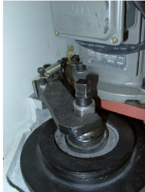
Figure 5.7 – Spindle lock fork engaged
