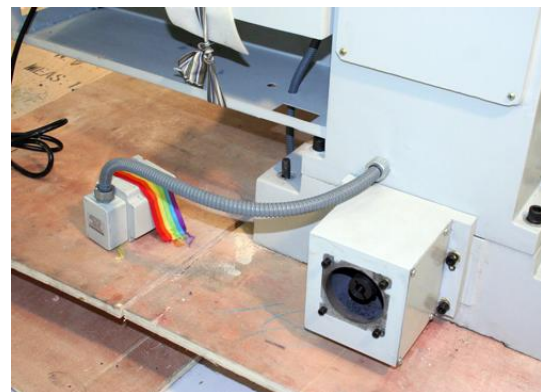
Figure 2.5 – Y-axis motor as shipped and mounting flange
