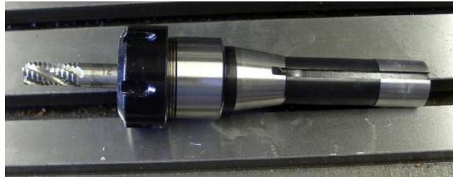
Figure 5.6 – ER32 collet tool holder
