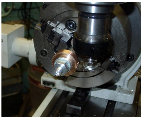
Figure 8.4 – Gear cutting (tailstock removed for clarity)
