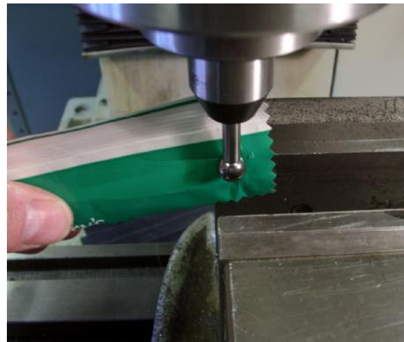
Figure 6.22 – Measuring vise jaw Y position
