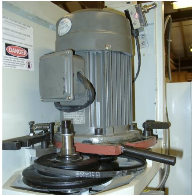
Figure 2.17 – Changing spindle pulleys
