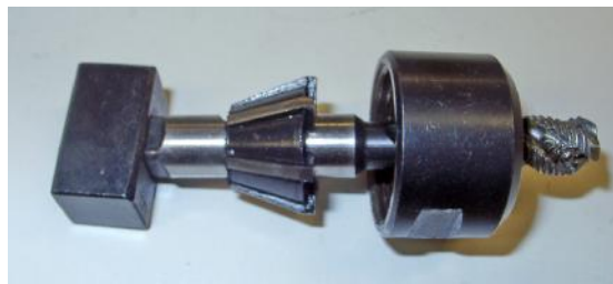
Figure 8.24 – Tap collet and anti-rotation block
