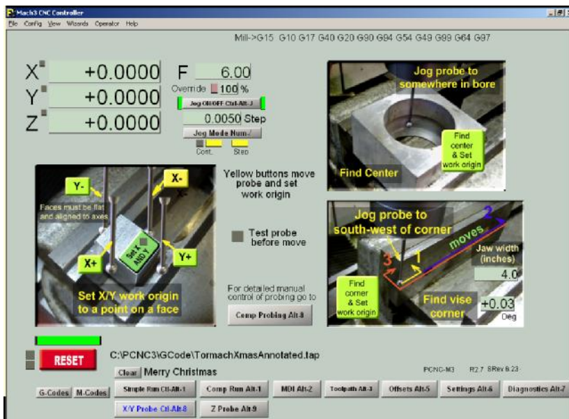
Figure 8.10 – Simple XY Probing
