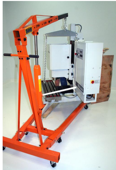
Figure 2.7 – Hoist bar for slinging the mill
