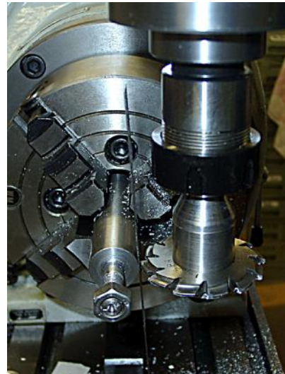
Figure 8.6 – Ruler tilted to left at top so cutter is too high
