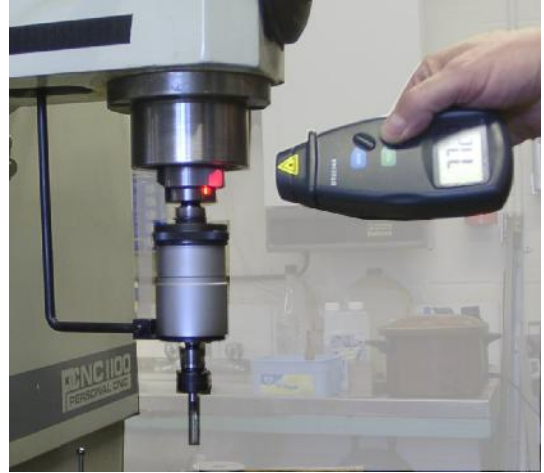
Figure 8.27 – Measuring spindle speed
